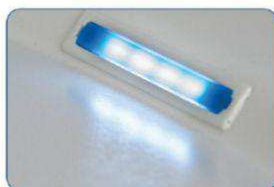
Visual signal of end of centrifugation
